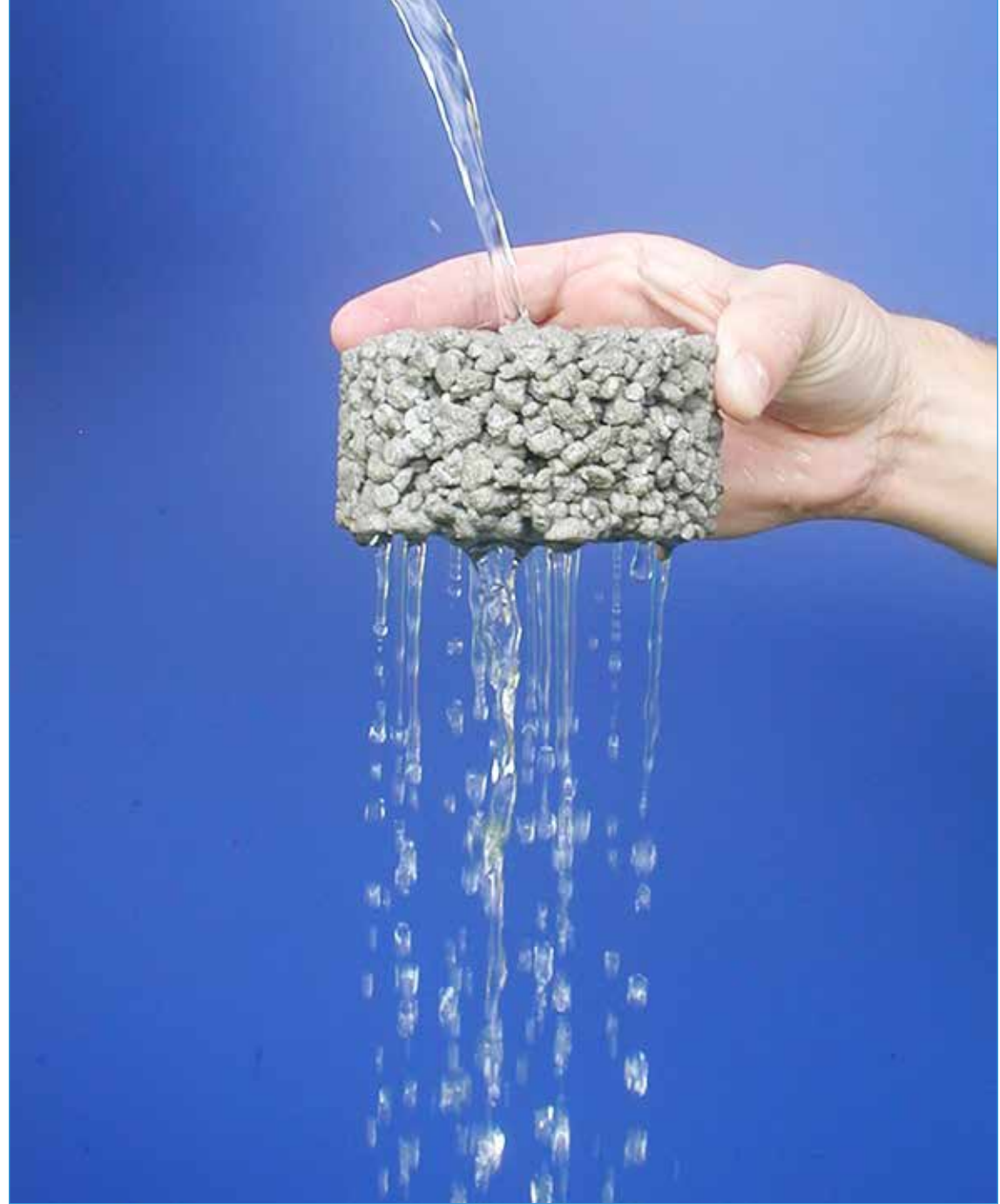
Figure 7.6: Pervious pavement keeps water from accumulating and thus can help prevent falls.
