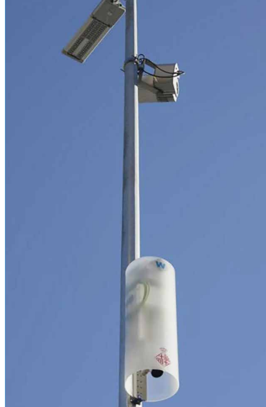
Figure 10.10: Digital sensors enclosed within plastic cylinders on light fixtures can measure light intensity, temperature, sound, or air quality and transmit that data for analysis.
