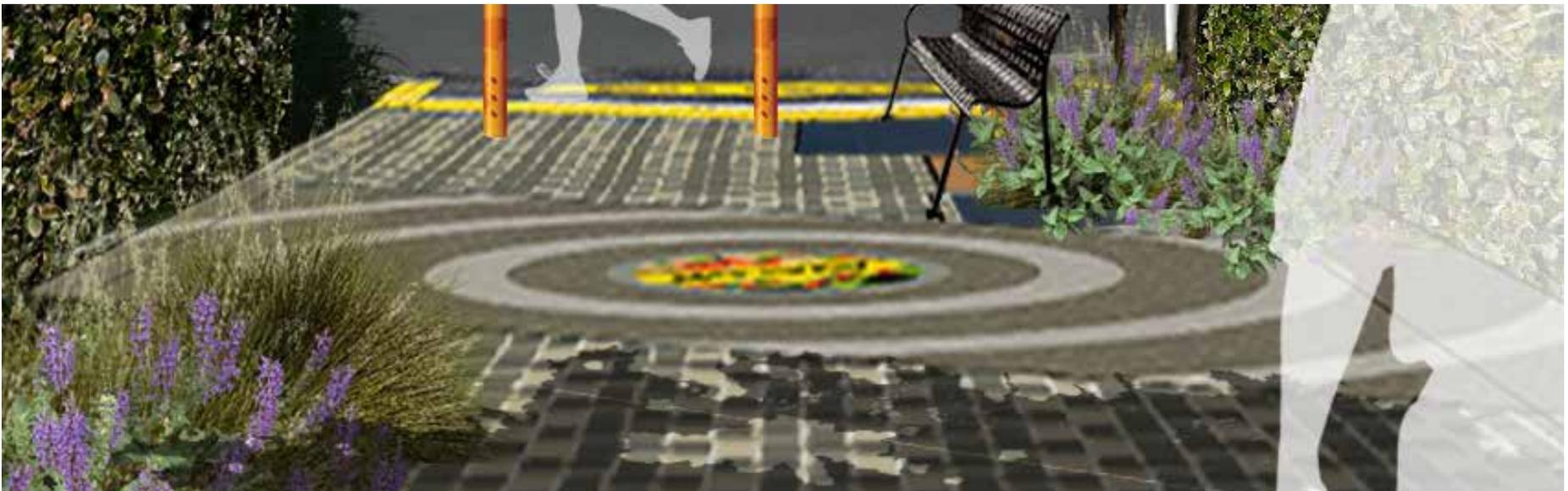
Figure 38: Conceptual rendering of the Avalon Project's permeable paving and catch basins
