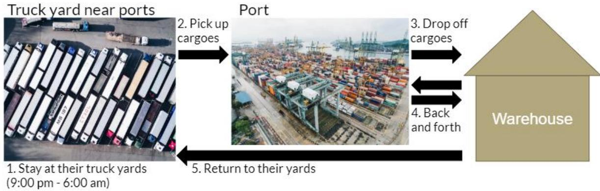
Figure 7. Drayage Truck Duty Cycle
