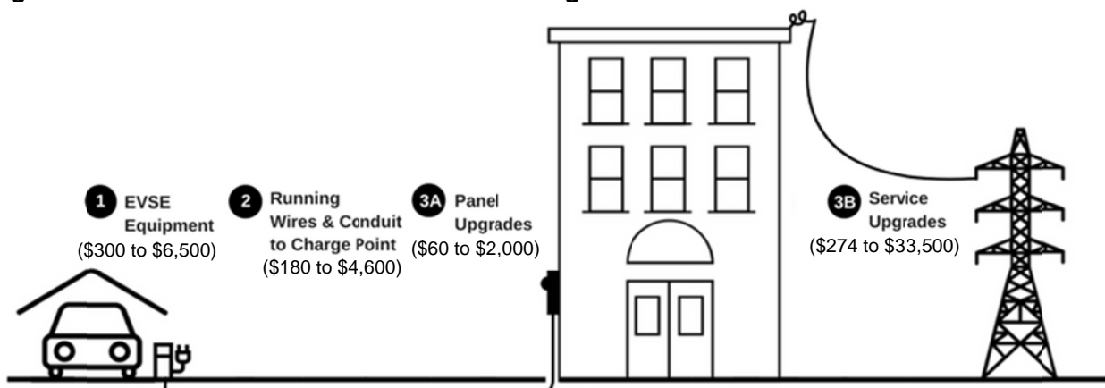
Figure 4.1: Potential Costs at the Different Stages of EVSE Installation at MUD Locations
