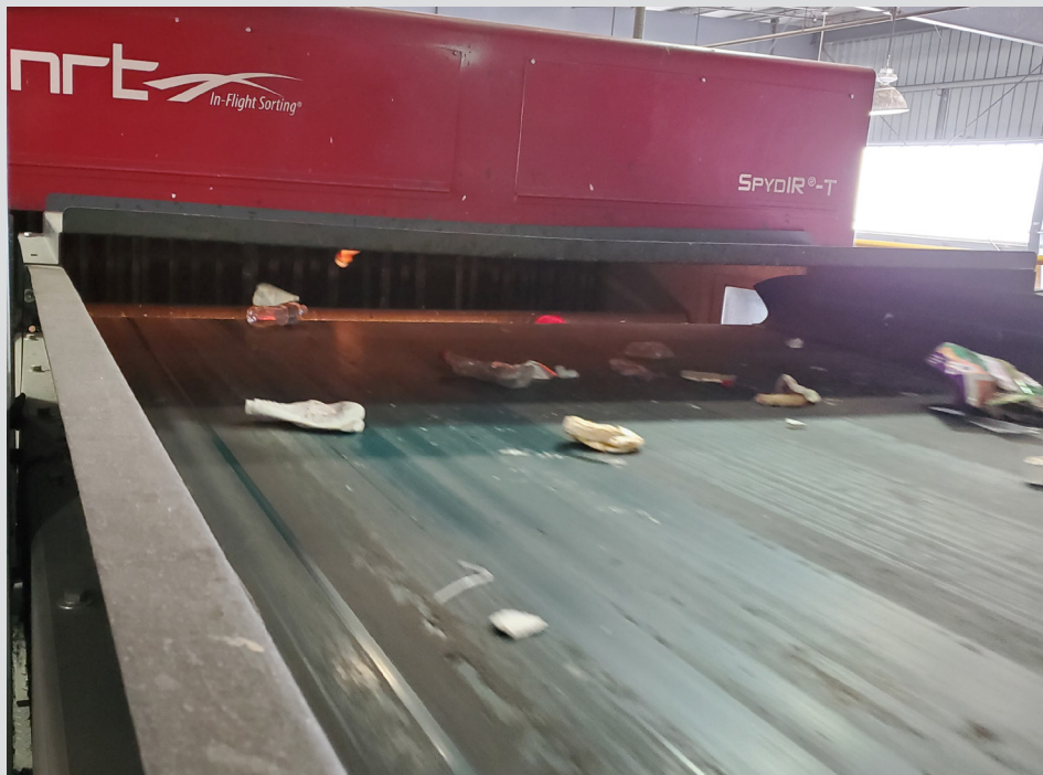
Figure 1: An optical sorter at work.
