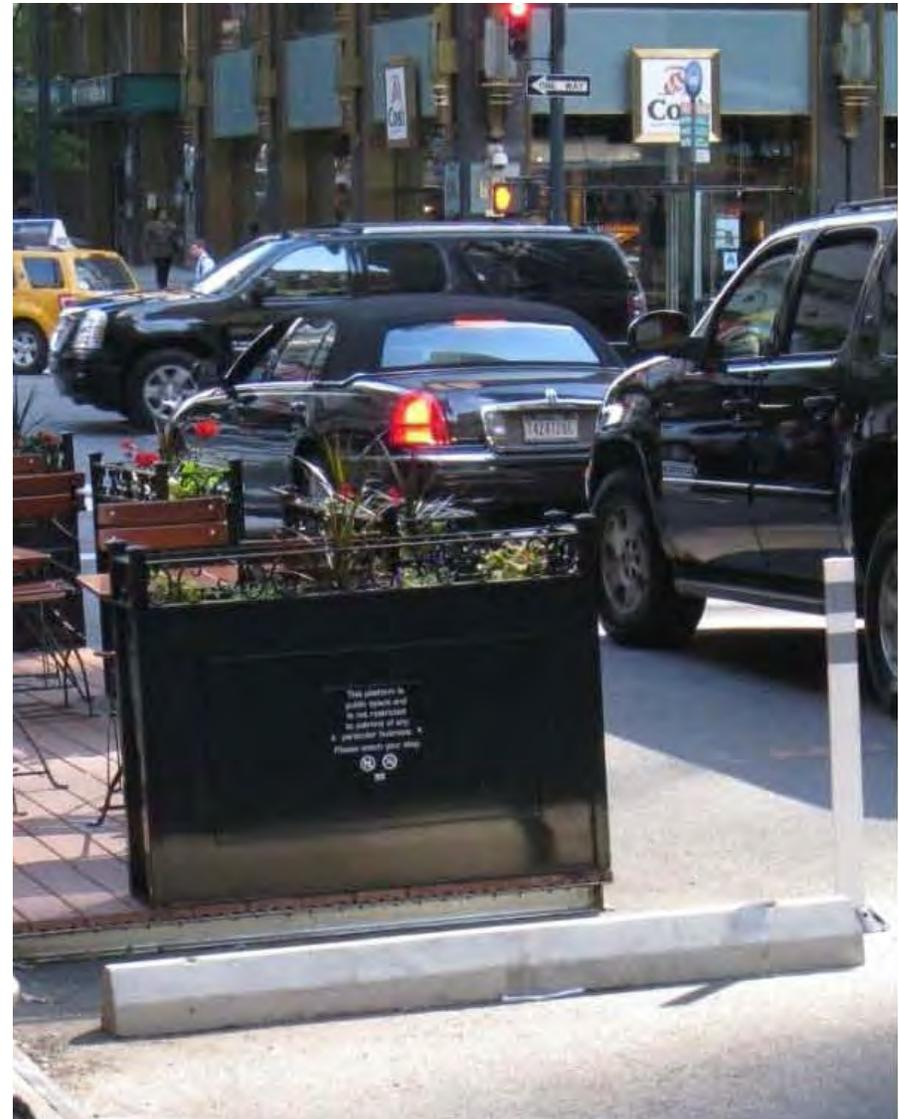
*Figure 41.* Flexible bollard and wheel stop, New York City, NY.
