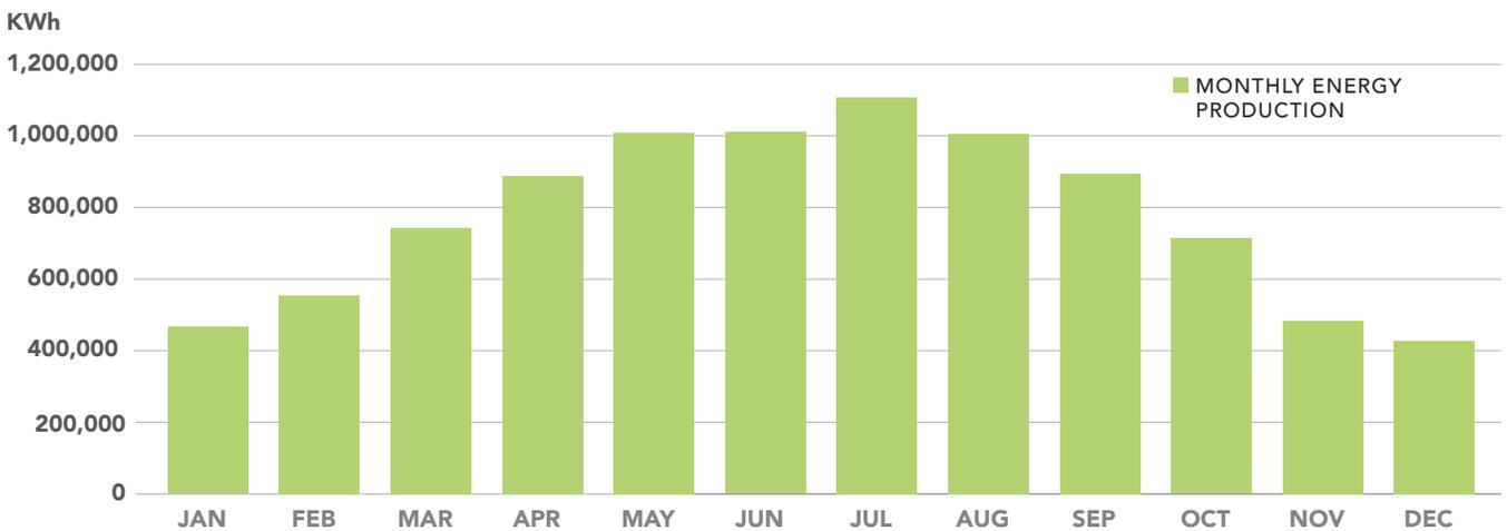
**FIG 12** Electricity generation from all MCE’s FIT installations
