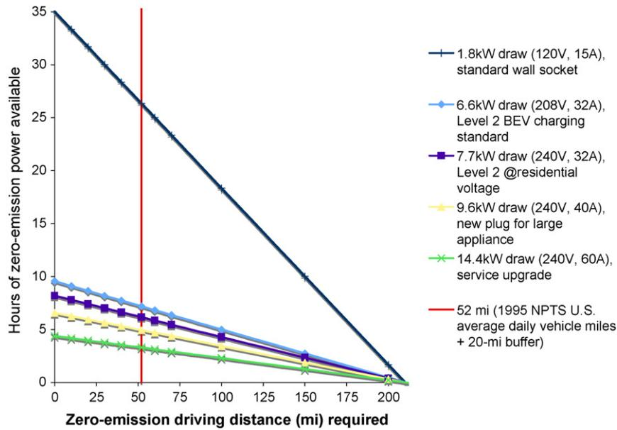
Fig. 2. Zero-emission Mobile Electricity vs. zero-emission driving: FCX 2006.
