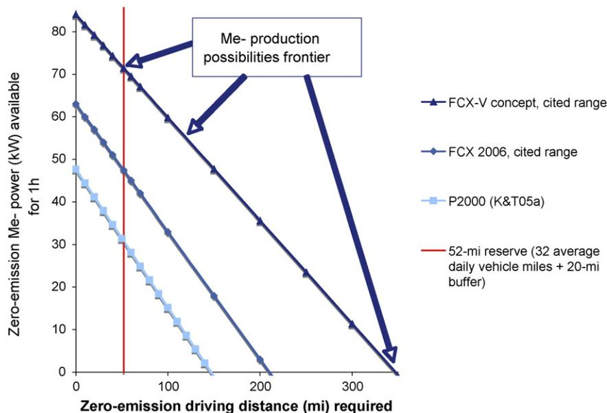
Fig. 6. One-hour power capacity vs. driving distance for various FCVs.
