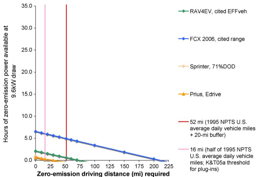
Fig. 4. Zero-emission Mobile Electricity vs. zero-emission driving: 9.6 kW load.
