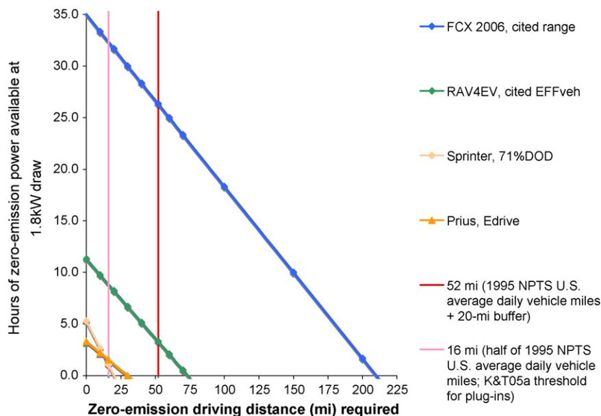
Fig. 3. Zero-emission Mobile Electricity vs. zero-emission driving: 1.8 kW load.
