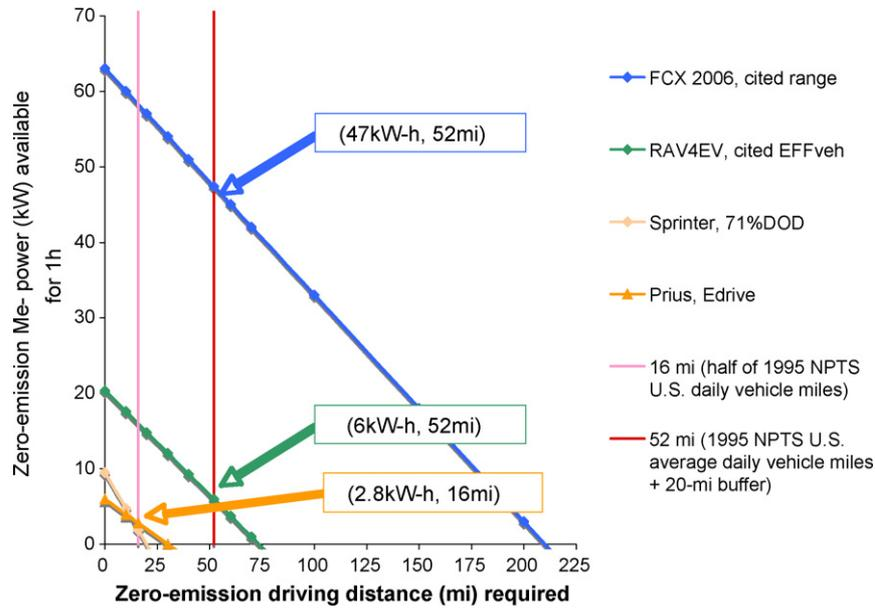
Fig. 5. One-hour zero-emission power capacity vs. zero-emission driving distance.
