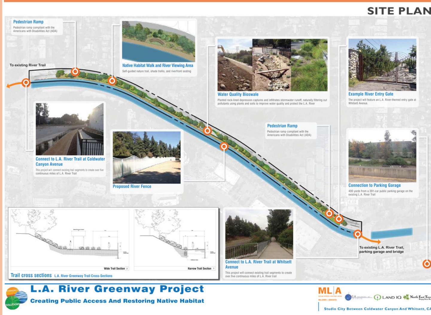
Figure 4 – 23: Site plan showing the location of bioswales, pedestrian ramps, and other project features.
