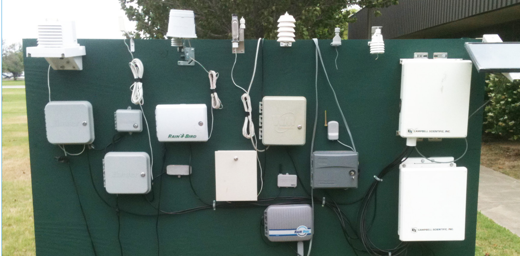
Figure 5.3: Smart controllers adjust watering cycles using data from ground and weather sensors. The rectangular boxes are controller programming units; the non-rectangular pieces mounted on top of the green panel are weather sensors.
