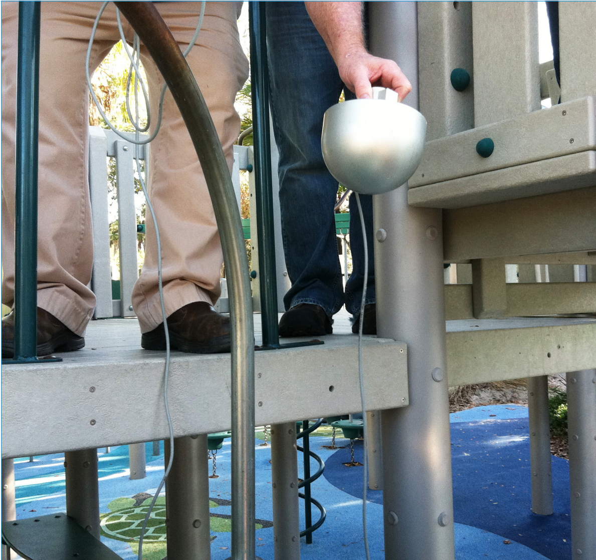
Figure 8.17: Hard-surface testing equipment is dropped off a play structure to mimic a child's head during a fall.
