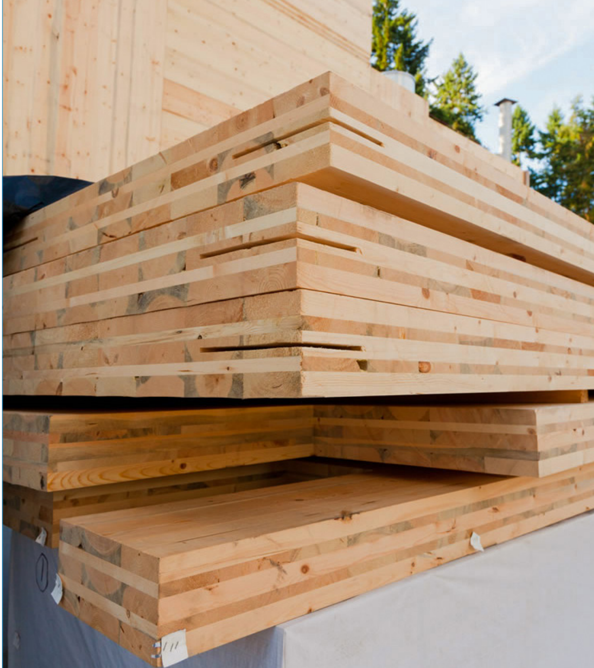
Figure 7.3: Cross-laminated timber, created from the waste of wood mills that would otherwise be discarded, helps reduce the carbon footprint of both the original wood product and itself.
