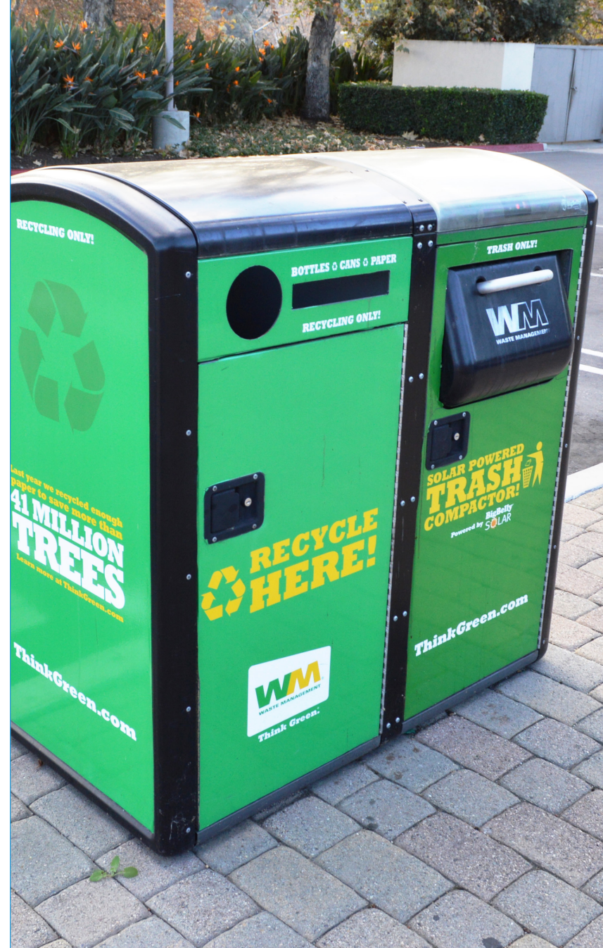
Figure 9.8: Solar-powered trash compactors like these on a Mission Viejo, California, street require less maintenance than traditional cans or bins.
