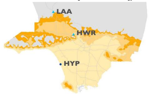
Each colored area represents a pumping extent for net-neutral energy use when displacing a supply alternative with AWT. Dark Orange- Desalination. Medium Orange- SWP Imports, Light Orange- CRA Imports.
