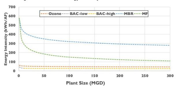
Figure 6: Estimated Energy Intensity Curves for Each Unit Process
