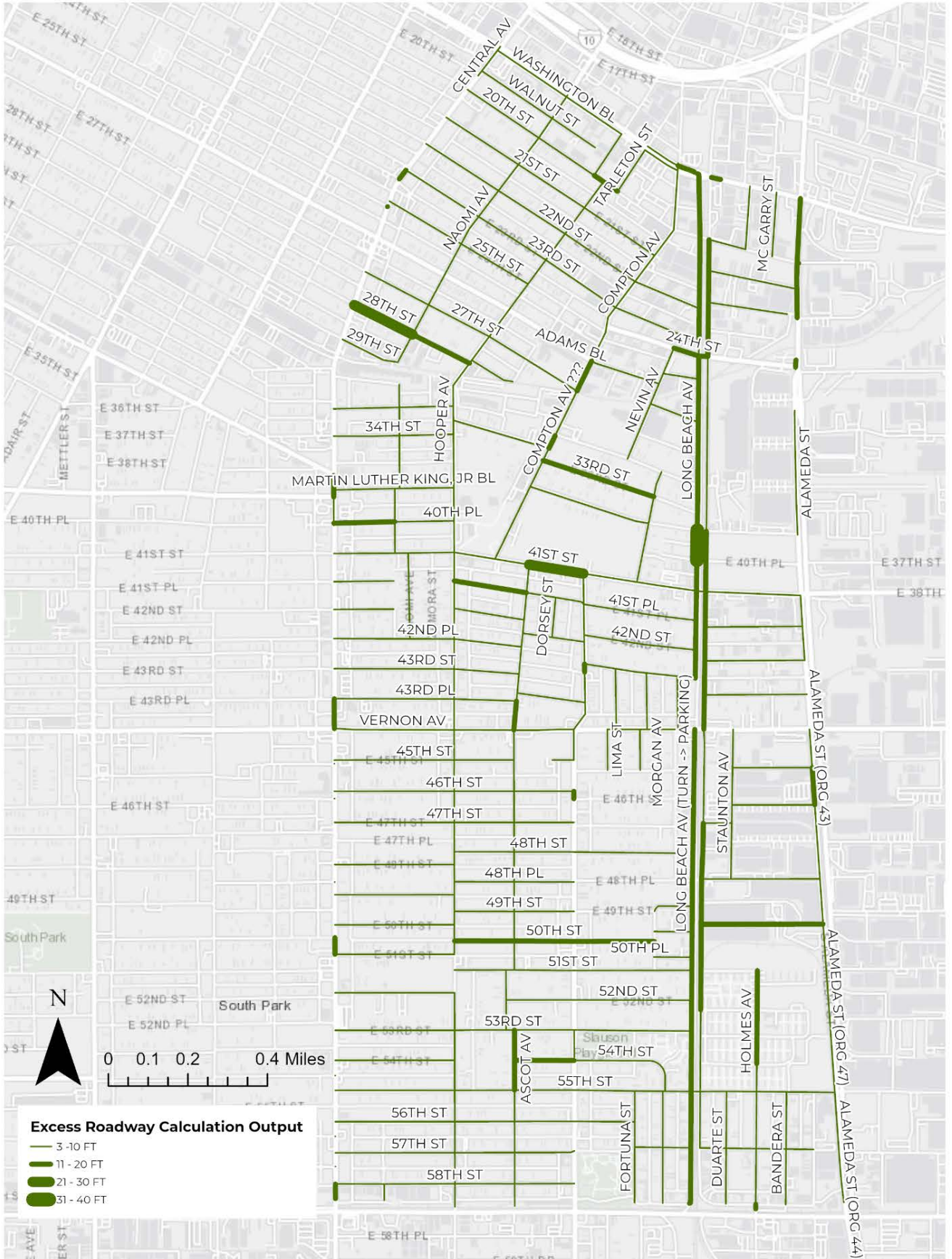
Figure 6. Central Alameda Total Excess Roadway Calculation Output
