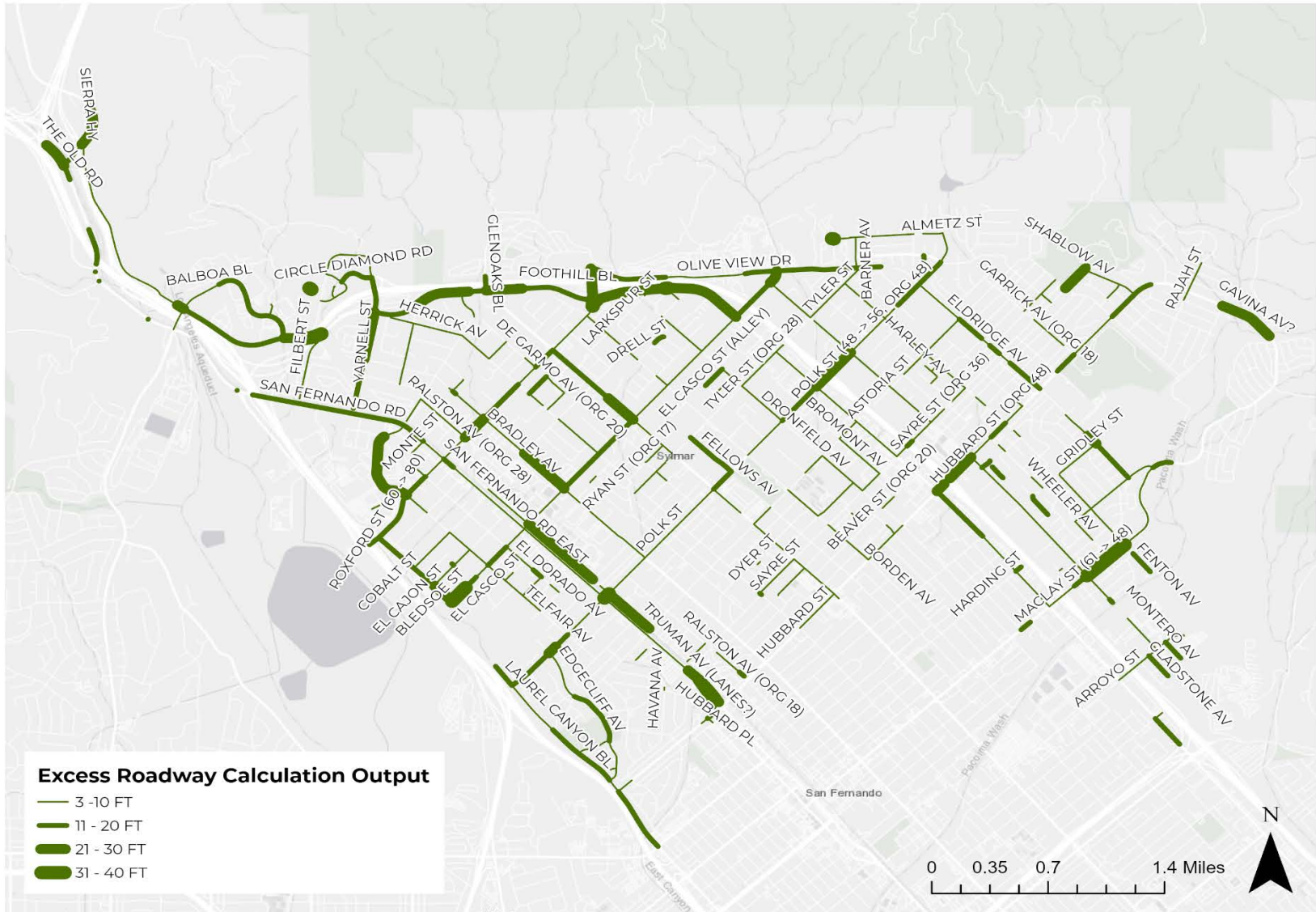
Figure 7. Sylmar Total Excess Roadway Calculation Output
