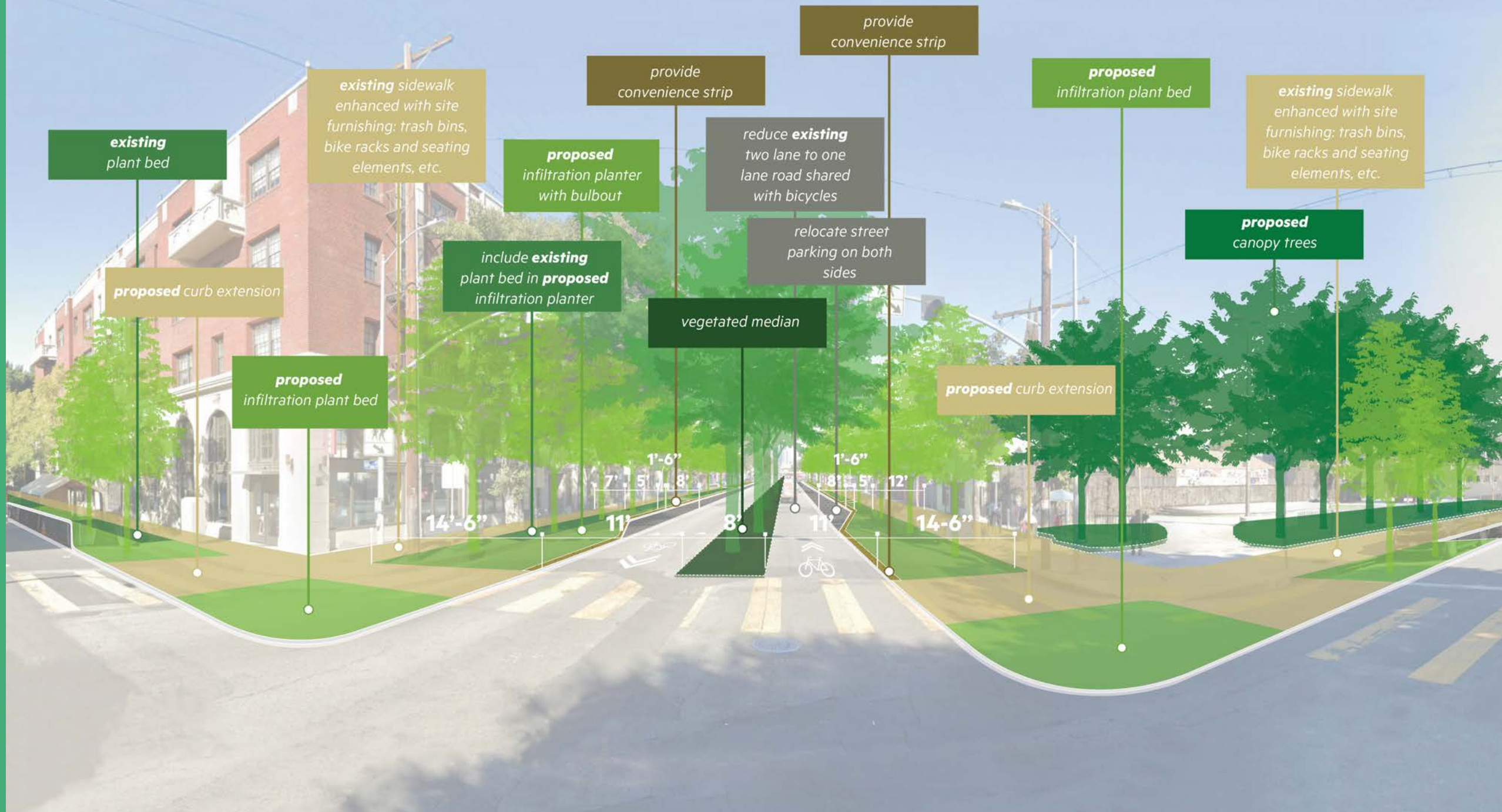
Figure 24. Central Avenue and 42nd Place, proposed design diagram, Tier 3 Credit: Stoss Landscape Urbanism
