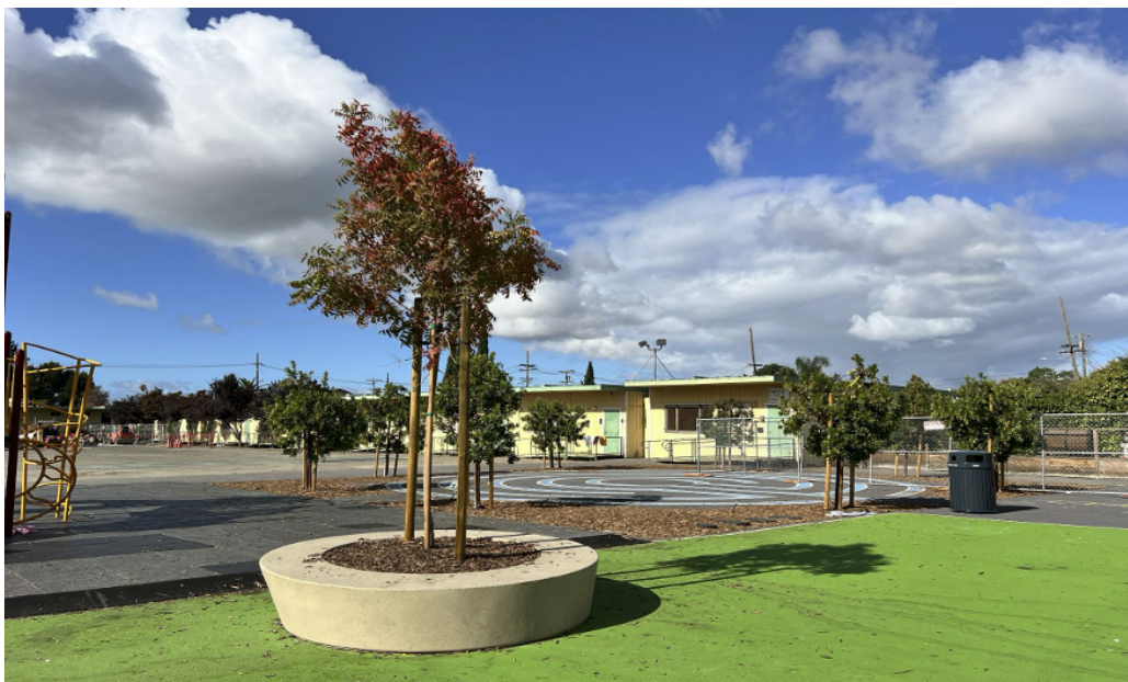
B. Portable classrooms behind a hardscaped playground area in East Oakland Pride Elementary School in OUSD, California. The new playground installation in 2024 involved depaving, strategic tree plantings, and painted asphalt to reduce albedo (sunlight reflected by the ground). Source: Levon Bigelow (2024)
